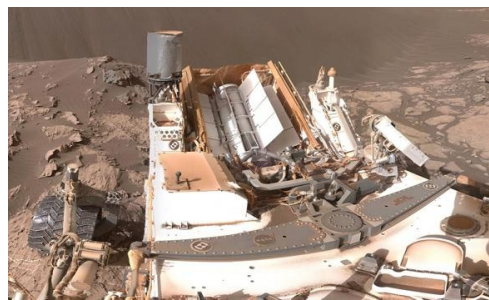
Figure 10. Multi-Mission Radioisotope Thermoelectric Generator on the Curiosity Mars Rover [79].
