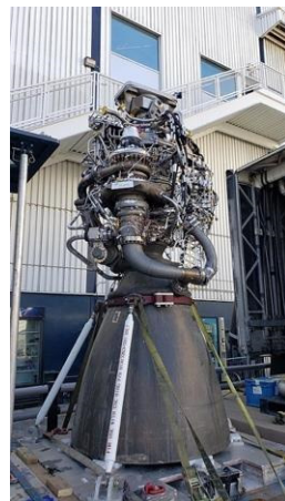
Figure 5. SpaceX's raptor engine, one of the first widely used LOX/methane engine [57].
