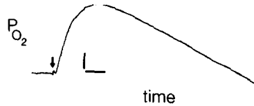
FIGURE 6. Time course of P_{O_2} in a chamber initially equilibrated with air, after a muscle equilibrated with 95% O_2 was placed in the chamber at time t = 0 , indicated by the arrow. Scale bars indicate 2.75 mmHg and 2 min. Extrapolation of the final linear phase of the record back to t = 0 gives an intercept \Delta analogous to that of Fig. 1C.
