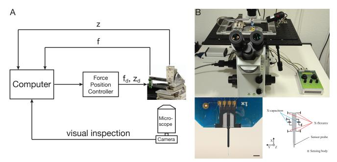
**Figure 1.** The cellular force microscope (CFM). (**A**) Schematic representation of the CFM. f and z are the measured values and  $f_d$ ,  $z_d$  are the desired values of force and position, respectively. (**B**) The CFM setup on an inverted microscope. The lower panels show an image of the MEMS-based force sensor on the left and a schematic on the right side. Scale bar = 1 mm. Images in (**B**) taken from [68].
