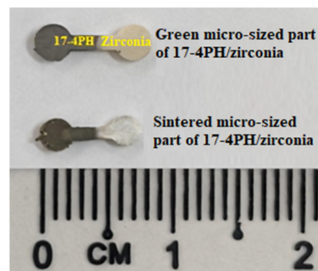
Figure 7. Photograph of green part and debound part sintered at 1350 °C.
