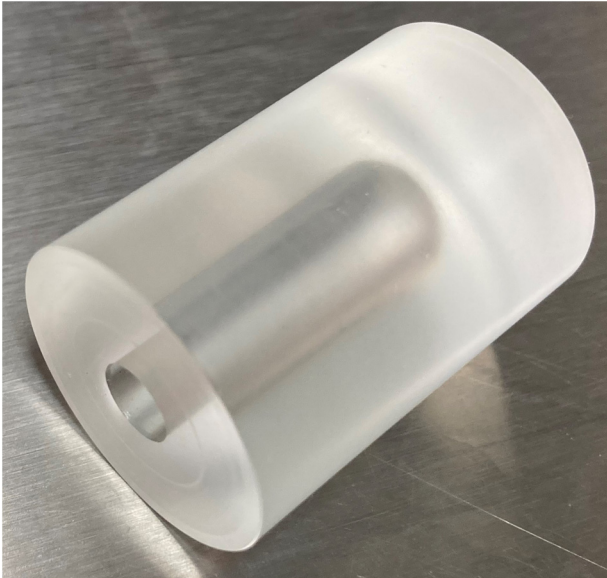
Figure 3. Cylindrical phantom. The PMMA phantom is used for the arc check. An ion chamber can be inserted to measure the dose in the center of the phantom.
