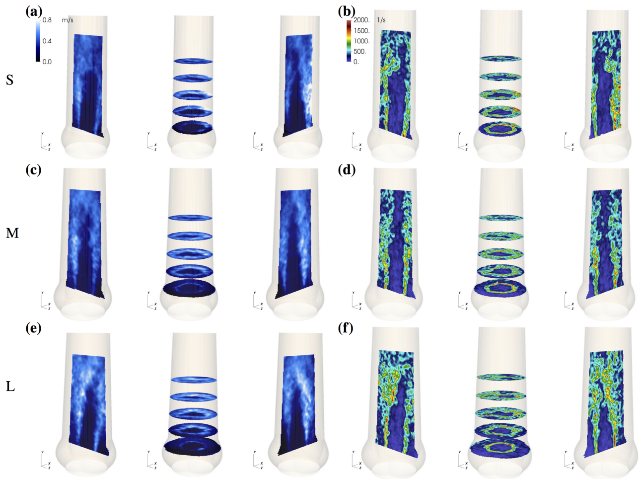
Fig 9. Properties of aortic jet shear layer. RMS velocity fluctuation field u_{rms} (a, c, e) and 3D shear rate \gamma_{3D} (b, d, f) at t = 0.21 s for small (S), medium (M), and large (L) aortic root size.
