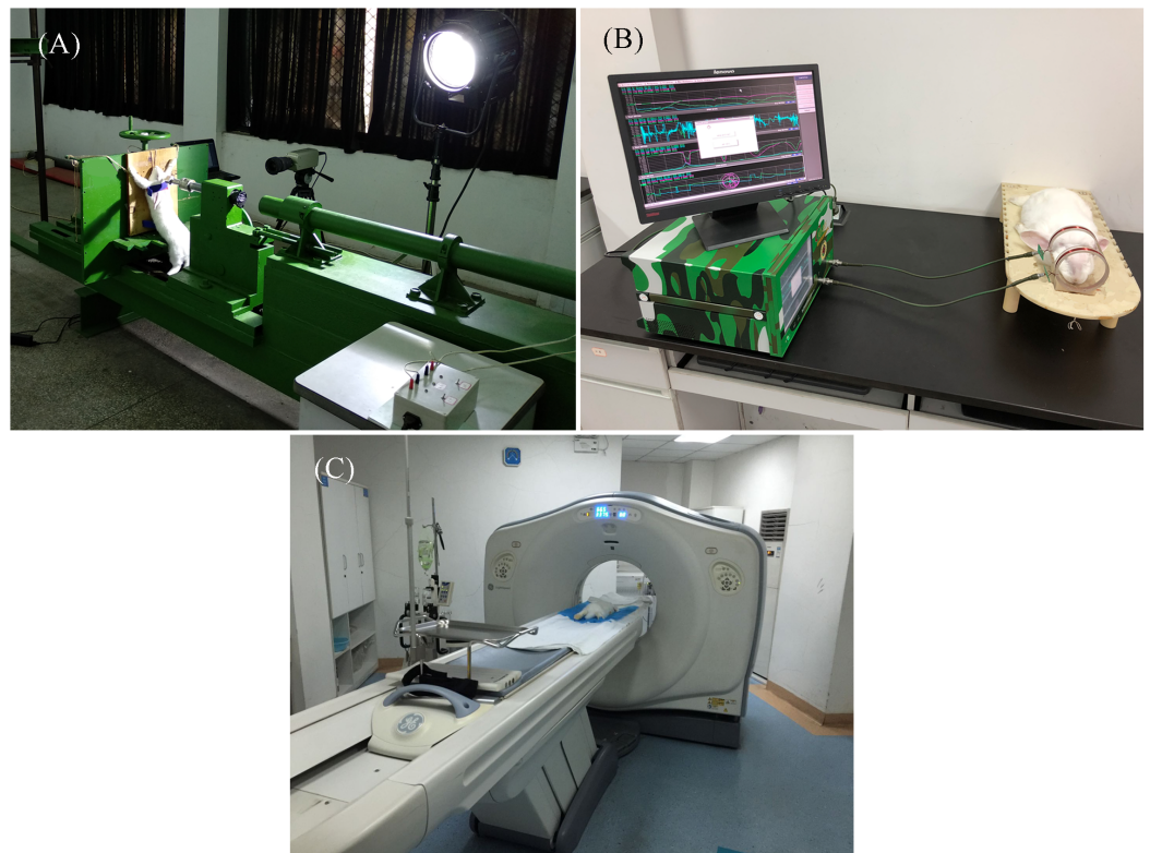
Figure 4 Experimental setup of CCH. Horizontal biological impactor BIM-II (A). CCH detection system in rabbits (B). CT image acquisition of a rabbit (C). Photographs by Jun Yang.
