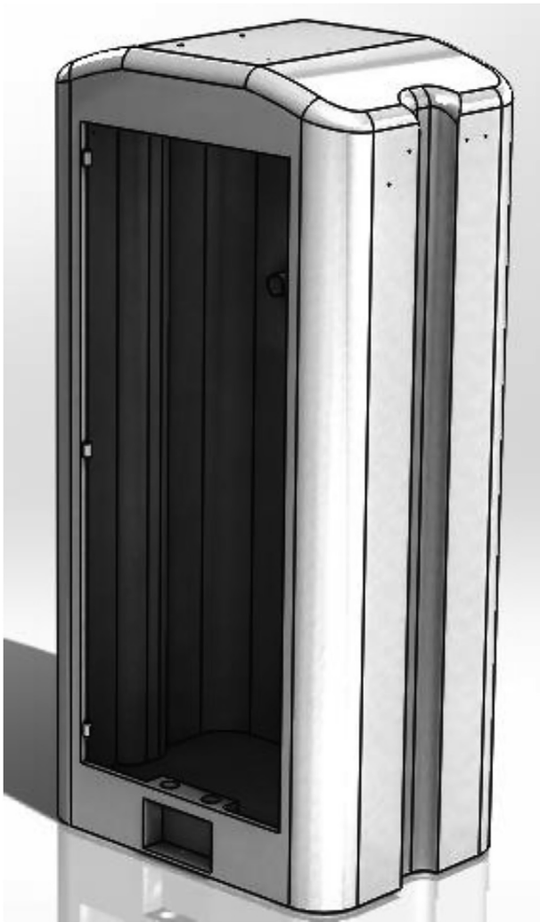
Fig. 8. Rearview which shows gate for ease of access and at the bottom, holes for attaching medical air hoses.
