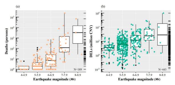
**Figure 6.** The relationship between *Ms* and earthquake-induced DELs (**a**) and deaths (**b**). The earthquake disasters plotted in the figures are associated with at least one death (**a**) or with reported DELs (**b**).
