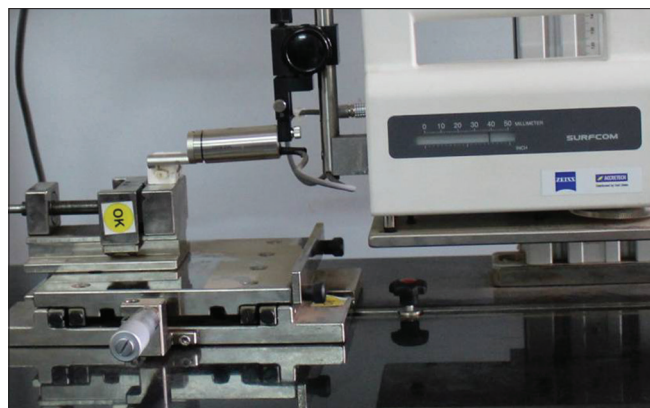
Figure 2: Profilometer (quantitative surface roughness evaluation of the prepared tooth)
