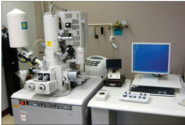
Figure 4: Scanning electron microscope (qualitative surface evaluation of the prepared tooth and the rotary diamond burs)
