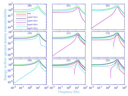
**Figure 6.** The total and individual energy in-flow transmissibility spectral densities into the vibration isolator bushings versus the frequency, at the force excitation points [n m], with n, m = 0, 1, 2.
