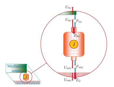
**Figure 2.** Displacements, forces and time averaged energy flows at the connecting surfaces to the mechanical source and to the infinite metal foundation for the vibration isolator bushing (j), where j = 1, 2, 3, 4.
