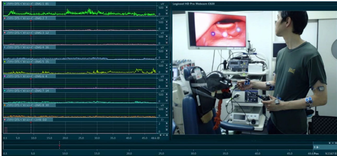
FIGURE 4 Surface EMG recording during the NPE tasks. Simultaneous recording of sEMG in the targeted eight muscles of the participant was performed during NPE tasks performed on a training model set on a treatment chair. NPE, flexible nasopharyngeal endoscopy; sEMG, surface EMG
