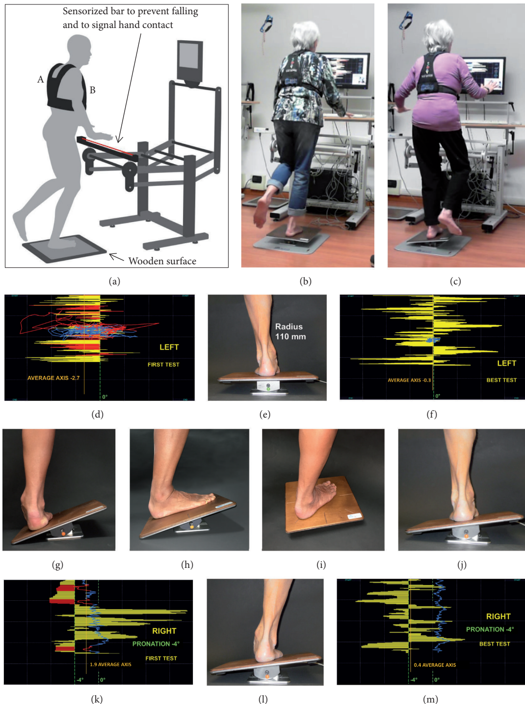
FIGURE 1: (a) The postural proprioceptive station [17]. The red line represents the infrared ray of the sensorized bar. Vest (A) to support the “postural reader” in (B) sternal position. (b, c) A subject on the electronic rocking base in single stance during a training session. (d) The real-time trace (yellow bars) of the rocking base (e) and the trace of the postural reader (blue line). Note the presence of precautionary strategy (red trace) and hypersupination in the first test (d) vs. the best test (f). (g, h) Static exploration of the ankle range of motion: maintaining vertical stability with the weight-bearing ankle in hyperpronation and in maximum dorsiflexion. (i) Orientation of the rocking base at -45^\circ to affect different ranges of motion. (j, k, l, m) Dynamic exploration of the ankle range of motion: (j) supination (inversion); (k, l, m), attempting to maintain 4^\circ of inclination (pronation, eversion). All subjects were asked to minimize postural instability (blue line).
