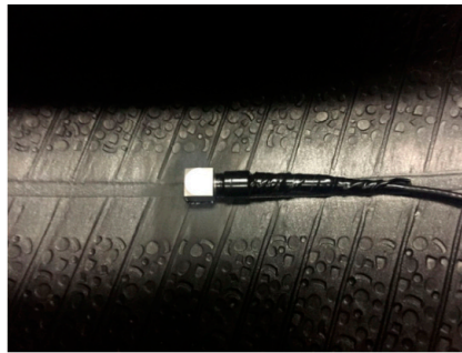
Figure 7. Tri-axial accelerometer tread sensor [23]. Reprinted with permission from [23].
