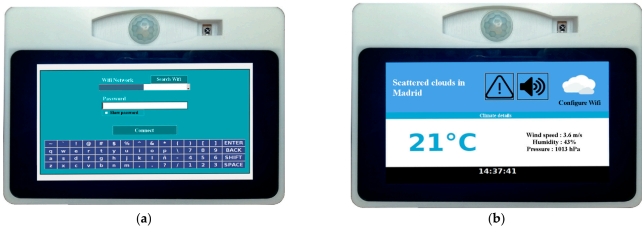
Figure 4. (a) Screen to configure the Wi-Fi network of the house; (b) Screen to check the current weather.
