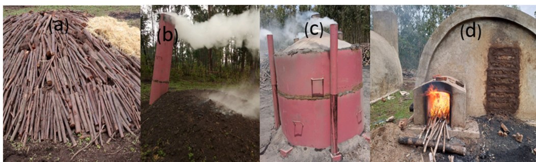
Fig. 3. The different charcoal production technology used in the study: Earth mound kiln (a), Casamance (b), MRV steel (c). Green mad retort (d). Photo credit researcher, (2022).
