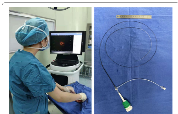
Fig. 1 Photograph of OCT system used in the study and its catheter probe
