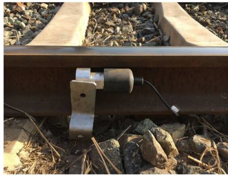
Figure 15. Installation of ultrasonic transducer at rails.
