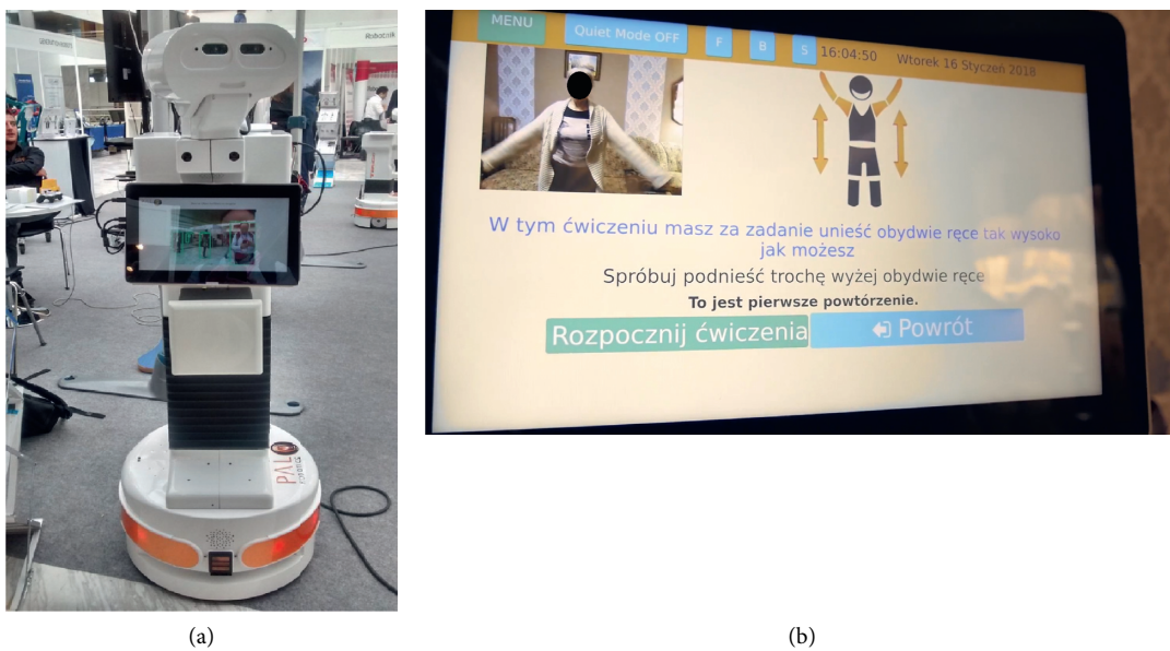
FIGURE 8: ENRICHME interactive mobile robot (a) and its service of physical exercise monitoring (b).
