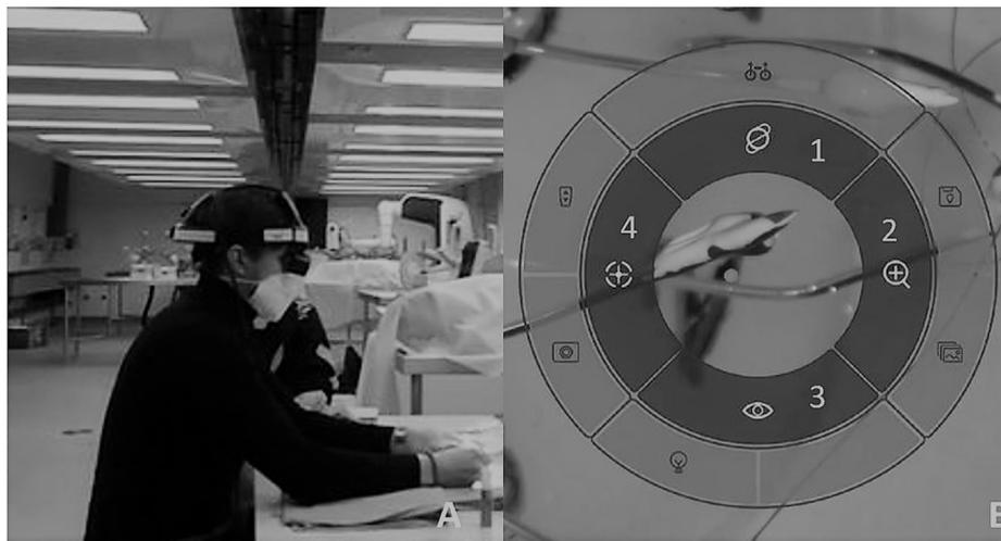
**Fig. 1.** Start position of the participant with HMD set up and exercise centered on the working table (A). Operating the robot controlled exoscope with the user interface (B, 1 = orbit movement, 2 = magnification, 3 = translating movement, 4 = focus).
