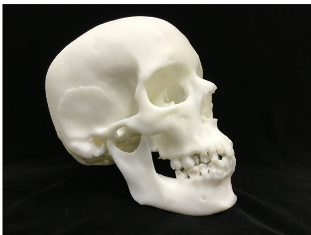
Fig. 12 3D-printed skull extracted from a CT scan using FDM printing
