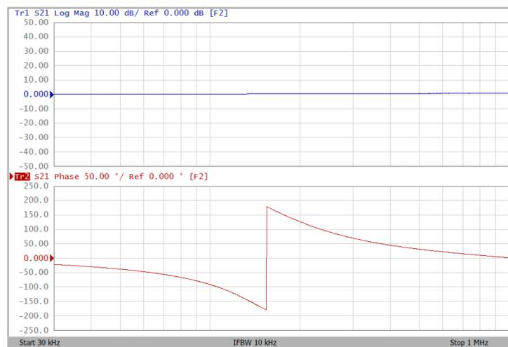
Figure 23. Experimental results of gain (blue) and phase (red) responses for AP filter at  $V_{O3}$  when  $\pm 2$  V DC supply.
