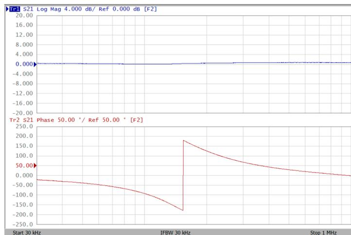
Figure 15. Experimental results of gain (blue) and phase (red) responses for AP filter at  $V_{o3}$  with  $V_{i1} = V_{i2} = V_{in}$ , and  $V_{i3} = V_{i4} = V_{i5} = 0$  when  $\pm 15$  V DC supply.
