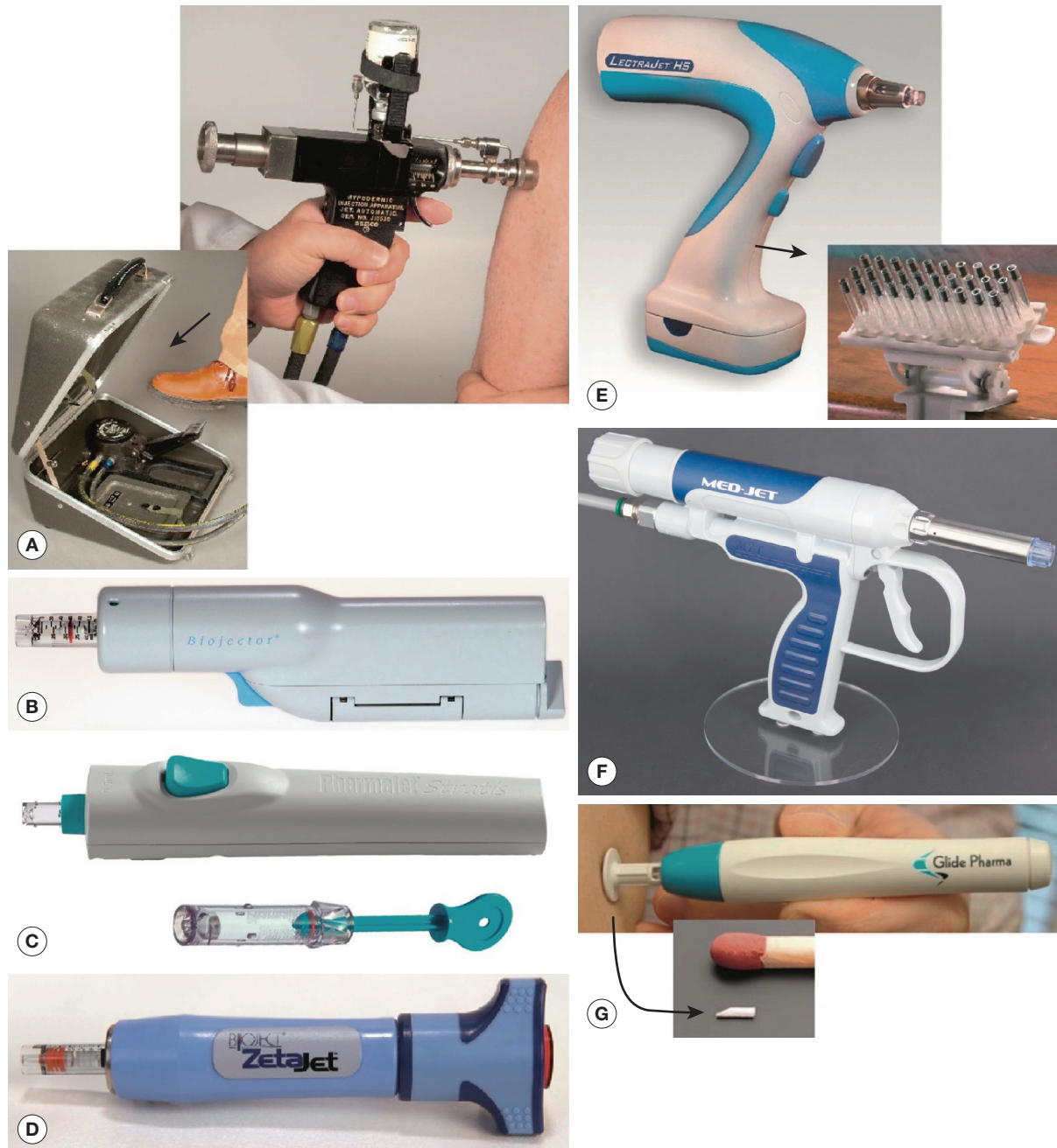
Figure 68.4. Selected devices for subcutaneous and intramuscular vaccine delivery. A , Ped-O-Jet (Keystone Industries), the most widely used multiuse nozzle jet injector (MUNJI) worldwide, before withdrawal from public health use by the 1990s for cross-contamination risk. Its metal spring is compressed by hydraulic fluid pumped by a foot pedal in its carrying case ( A , inset) or by electric pump (not shown). Depth of delivery determined by removable nozzle used, either a subcutaneous (SC)/IM nozzle (shown here) or an intradermal (ID) nozzle (see Fig. 68.3E). B , Bioject 2000 DSJI, powered by gas. It has Food and Drug Administration (FDA) clearance for SC, IM, and ID delivery. C , PharmaJet Stratis DSJI, for 0.5-mL dose delivery. Delivery IM or SC set by vaccinator technique (fat layer pinched up for SC). Spring is reset using separate carrying case. Syringe is filled by pulling back and breaking off its blue shaft and thumb tab from conventional single-dose and multidose vials using needle-free vial adaptor (not shown). On insertion into device, any excess liquid is returned to vial to minimize wastage of overfill. Cleared for U.S. marketing by the FDA in 2011 and received World Health Organization (WHO) prequalification in 2013. 715,716 D , Bioject ZetaJet metal-spring-powered DSJI, features built-in crank for manual recocking of metal spring (Bioject Medical Technologies). Uses different autolisabling cartridges for SC, IM, and ID injections (SC and IM delivery was licensed by U.S. FDA in 2009; ID use is investigational). E , Investigational LectraJet HS (high-speed) motorized DSJI (D'Antonio Consultants International) features built-in motor and rechargeable battery for rapidly compressing metal spring between injections at rates exceeding 600 per hour, with battery capacity of >3000 injections per charge. Capable of rapid loading and unloading of single-use syringes from ( E , inset) a sterile-packaged, 30-unit magazine for mass vaccination. F , Med-Jet H4 DSJI (Medical International Technology), gas-powered with entirely disposable single use fluid path. Licensed in Canada in 2014. A manually powered DSJI, the Dart (not shown), is in development and uses the same disposable cartridges. G , Investigational Solid Dose Injector (SDI) from Glide Pharma is powered by a compressed metal spring, which is released as the disposable drug cassette (white component extending beyond blue hub) is pressed fully against the skin. It inserts a ( G , inset) pointed, hardened, approximately 1-mm-diameter drug formulation (shown compared with conventional matchstick tip) into subcutaneous tissues, where it dissolves. ( A and inset, Courtesy James Gathany, Greg Knobloch [CDC Photographic Services]. B and D , Courtesy Bioject Medical Technologies. C , Courtesy PharmaJet, Inc. E , Courtesy D'Antonio Consultants International, Inc. F , Courtesy Medical International Technologies [MIT Canada] Inc. [Karim Menassa]. G , Courtesy Glide Pharma.)
