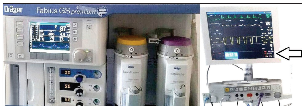
Figure 1: Erroneous display of halothane
