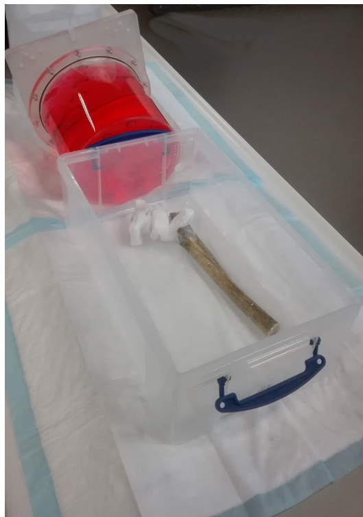
Fig. 3 Experimental setup. The picture shows the femur-implant assembly in the container not yet filled with water. Note the tape securing the sources in place. The scatter phantom is placed in front
