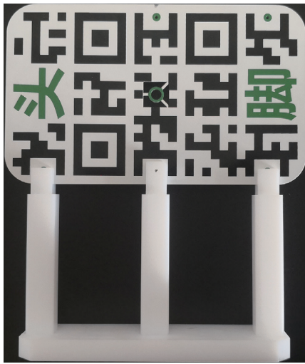
Figure 3 Positioning QR code. A board with a printed QR code, together with green head/feet direction indication letters (in Chinese). This board will be placed beside the operating area before navigation start. QR code, quick response code.
