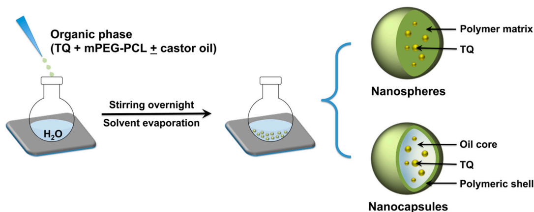
Figure 1. Overview of TQ NP fabrication by nanoprecipitation using mPEG-PCL. Different formulations were prepared by varying the MW of the PCL block with or without the addition of castor oil to the organic phase, which resulted in the formation of matrix-like nanospheres (NS) or reservoir-type nanocapsules (NC) with an oil-filled core and a polymeric shell.
