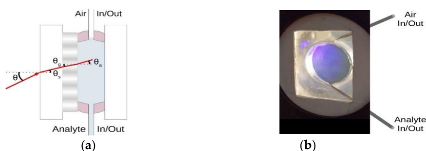
Figure 9. (a) Schematic sketch of the fluid cell with the beam propagation; (b) the image of the cell. Standard method: \theta = \text{constant} , \theta_a varies for different analytes. Modified method: \theta_a = \text{const} , \theta varies for different analytes.
