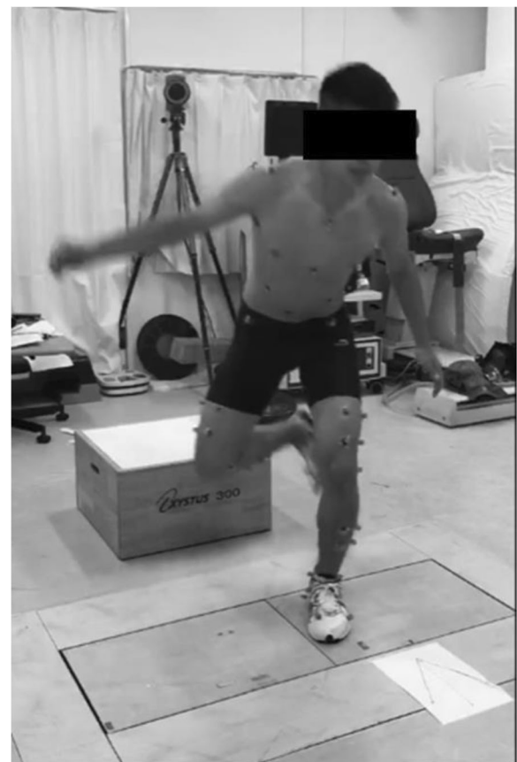
Fig. 2 Single-leg drop landing was performed for the non-dominant limb. Single-leg drop landing tasks were jumping from a 30-cm high box to a distance of 25% of their height away from the box, down to force plates
