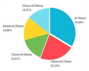
Figure 3. Coal gangue particle size distribution (mass).
