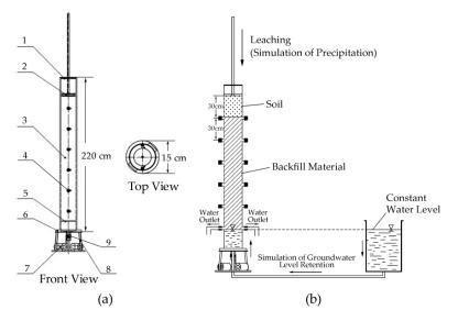
**Figure 2.** Testing Soil Column: (**a**) structure of soil column: 1-Testing soil column; 2-Piston rod assembly with graduated line; 3-Acrylic tube; 4-Angle valve; 5-Permeable tray; 6-Acrylic tube; 7-Balancing weight; 8-Base assembly; 9-Ball valve; (**b**) installation of soil column.
