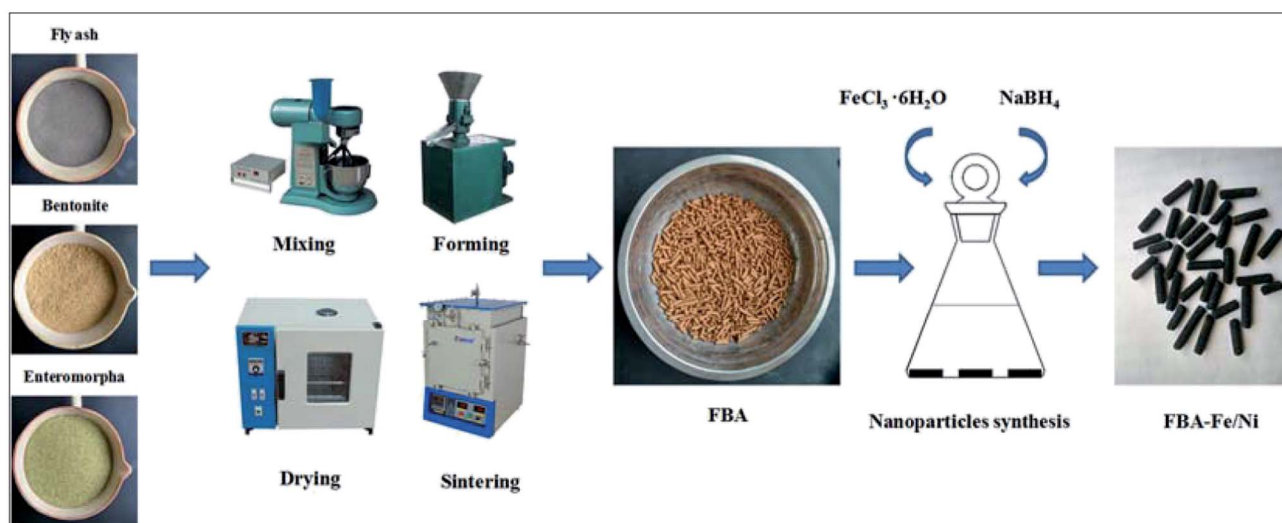
Fig. 1 Schematic diagram of FBA-Fe/Ni preparation.
