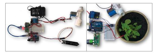
**Figure 4.** The IoT Object in the garden scenario is composed of an actuator for irrigation and sensors to measure soil's pH level, soil moisture, luminous incidence, and temperature.
