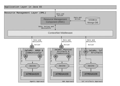
**Figure 5.** The technological view of components considering the IoT Objects employed in tests and the Engineering approaches in extended RMA.
