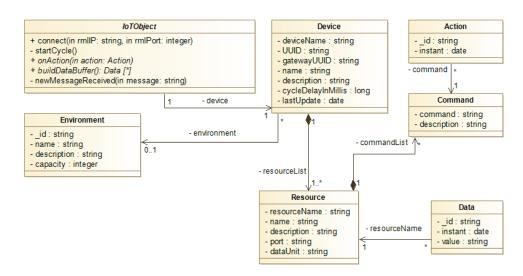
Figure 3. The extended RMA model.
