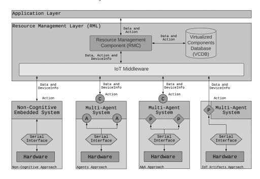
**Figure 2.** The extended Resource Management Architecture (RMA) and the three engineering approaches in the Device layer: the Agents, Agents and Artifacts (A&A), and the IoT Artifacts Approaches.
