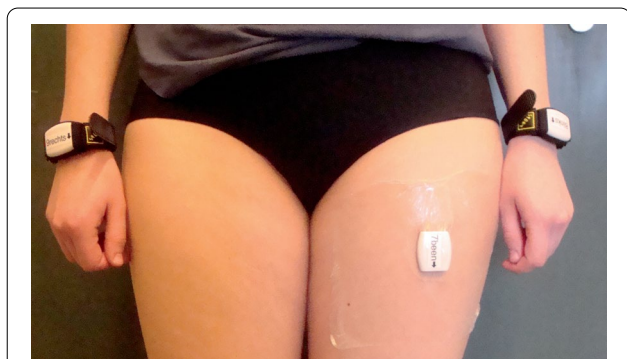
Fig. 1 The arm use monitor [7]. The system consists of two wrist-worn accelerometers and an accelerometer on the upper leg. The wrist-worn sensors measure arm movements and the leg sensor determines body postures and movements
