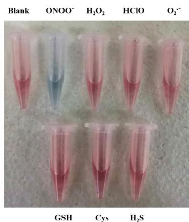
**Supplementary Figure 25** | Photos of HPQ-Zzh-B ( $20 \mu\text{M}$ ) to various analytes (1. blank, 2.  $5 \mu\text{M}$   $\text{ONOO}^-$ , 3.  $100 \mu\text{M}$   $\text{H}_2\text{O}_2$ , 4.  $50 \mu\text{M}$   $\text{HOCl}$ , 5.  $20 \mu\text{M}$   $\text{O}_2^-$ , 6.  $3 \text{ mM}$  GSH, 7.  $100 \mu\text{M}$  Cys, 8.  $100 \mu\text{M}$   $\text{H}_2\text{S}$ ).
