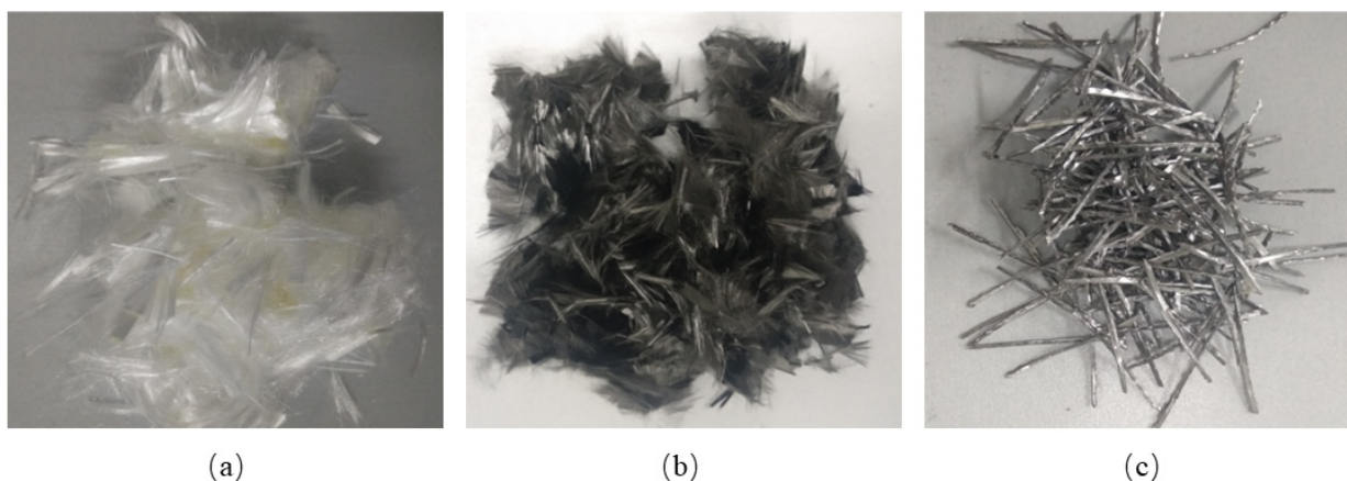
Figure 1. Fiber appearance. (a) PVA Fiber; (b) Carbon Fiber; (c) Steel Fiber.
