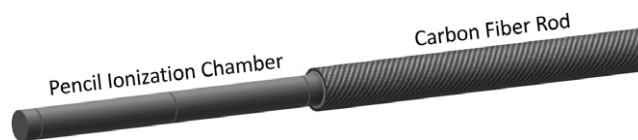
FIG. 2. This figure depicts how the pencil ionization chamber was attached to a carbon fiber rod so that measurements of CTDI_{free\ air} could be made.
