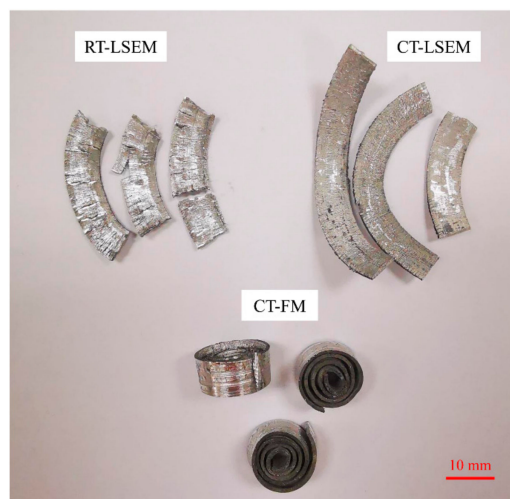
Figure 4. Chips and their morphologies of RT-LSEM, CT-LSEM, and CT-FM at a machining velocity of V_c = 5.4 m/min.
