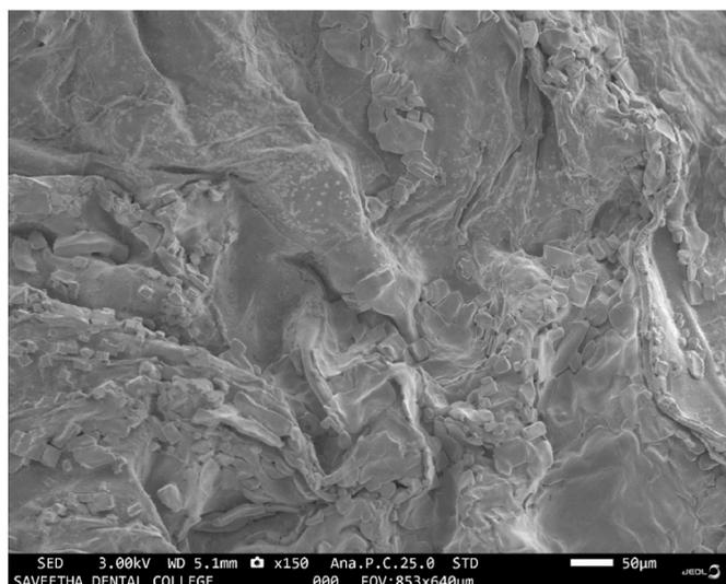
**Fig. 1.** SEM image of synthesized scaffold with *Cissus quadrangularis* extract, and tendon extracellular matrix (ECM).
