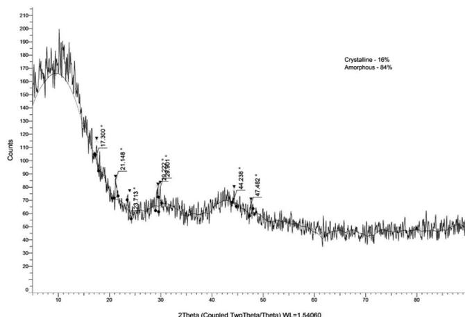
**Fig. 2.** XRD image of synthesized scaffold with *Cissus quadrangularis* extract, and tendon extracellular matrix (ECM).
