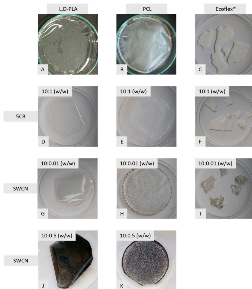
Figure 4. Photos of the created polymer layers by the drop-casting method: polymers L,D-PLA (A), PCL (B), Ecoflex ® (A–C), polymers with 5CB in a ratio of 10:1 ( w/w ) (D–F), polymers with SWCN in a ratio of 10:0.01 ( w/w ) (G–I), and polymers with SWCN in a ratio of 10:0.5 ( w/w ) (J,K).
