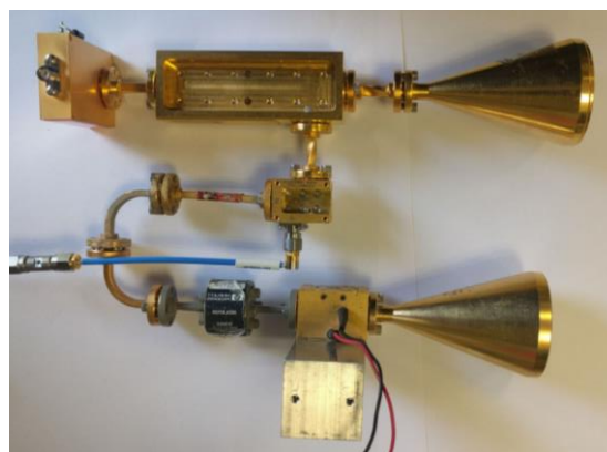
Figure 3. The continuous wave micro-Doppler radar.
