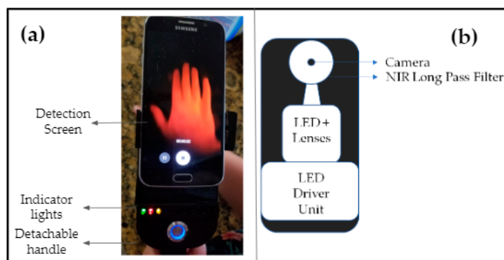
Figure 1. (a) Frontal view of the SPOT device, and (b) rear view with a custom attachment including all the imaging components, except the detector (which is the smartphone's camera).
