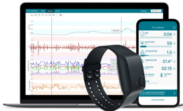
Figure 1. Empatica E4 Ecosystem implementing both computer (therapy management by the clinicians) and smartphone (data processing and display during patient use), retrieved from Reference [16].
