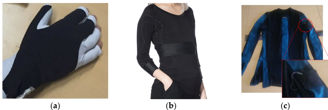
Figure 2. Different textile pieces integrating electronics for movement quantification in different areas of the body: (a) Glove for recognition of eight fundamental hand positions for Stroke patients [17]; (b) T-shirt to quantify symptoms of Parkinson’s Disease (PD), Epilepsy and Stroke patients [11]. (c) T-shirt to assess Stroke patients arm movement during daily activities [17].
