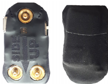
Figure 6. Hardware inertial unit coated with a slim, resistant textile.
