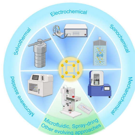
Fig. 2 Main methods for MOF synthesis. Solvothermal, microwave-assisted, sonochemical, electrochemical and mechanochemical synthesis are the most widely used methods, other methods such as microfluidic synthesis and spray-drying synthesis are also emerging and evolving
