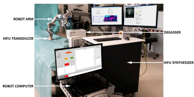
Figure 1 HIFU/DMUA set-up as used during a clinical procedure. DMUA, dual-mode ultrasound array; HIFU, high-intensity focused ultrasound.
