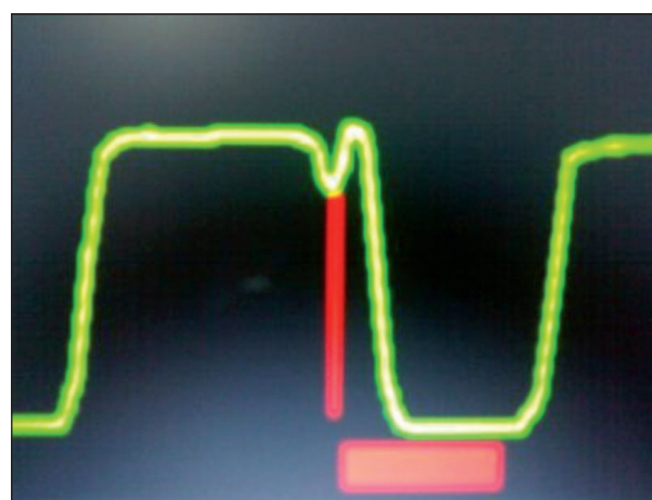
Figure 5: Sticking inspiratory valve – inspiratory flip – horizontal bar indicates possible rebreathing
