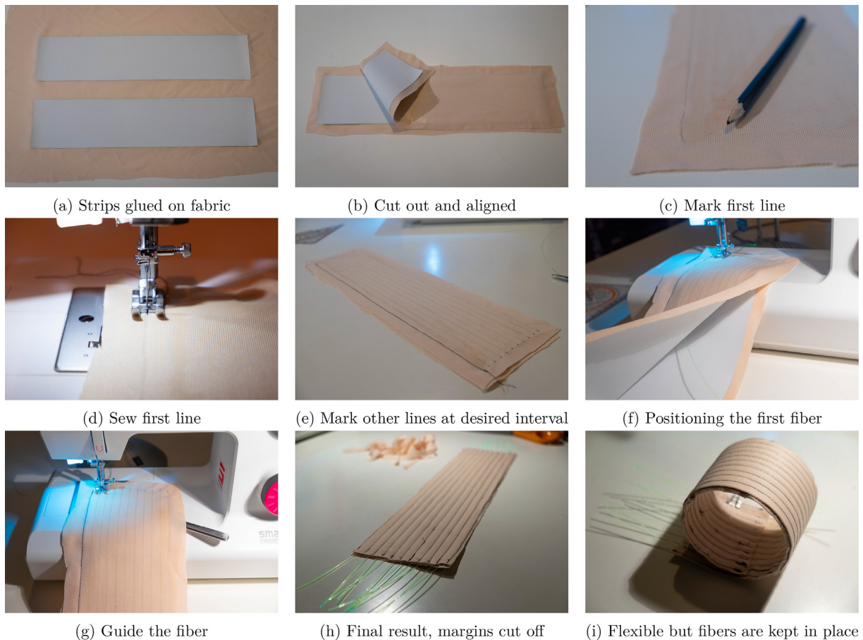
Fig. 4. Ribbon-detector Fabrication.
