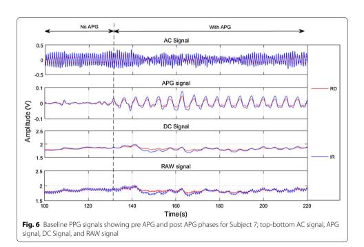
effectively constant since the APG system was not activated, while the AC signal pulsed due to the cardiac cycle. Upon activation of the APG system at approximately 130 s, the APG signal showed a period oscillation with an amplitude of up to 0.06 V.
