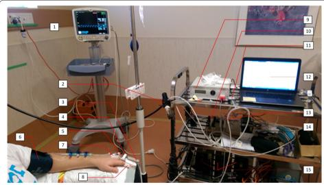
**Fig. 3** Typical equipment set up for this study. Key components are labelled. *1* dash monitoring screen, *2* air supply and regulator, *3* PO sensor, *4* thermocouple sensor, *5* digit pressure cuff, *6* blood pressure cuff, *7* venous line and catheter, *8* masimo SET sensor, *9* PO system, *10* solenoid vales, *11* pressure gauge, *12* PC running LABVIEW, *13* ITV001 pressure regulator, *14* NI DAQ system, *15* power supplies
