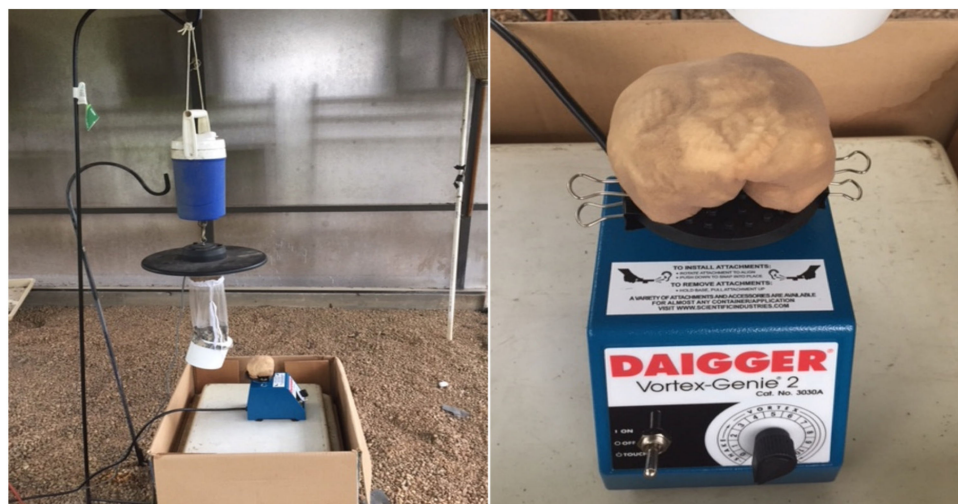
Figure 5. CDC trap and sheep wool placed in women's stocking attached to the Vortex platform head.
