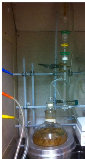
Figure 1. Hydrodistillation of sheep wool using the Clevenger type setup.
