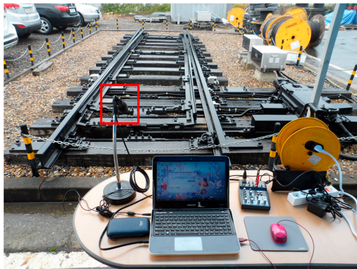
Figure 6. Data collection from NS-AM-type railway points.
