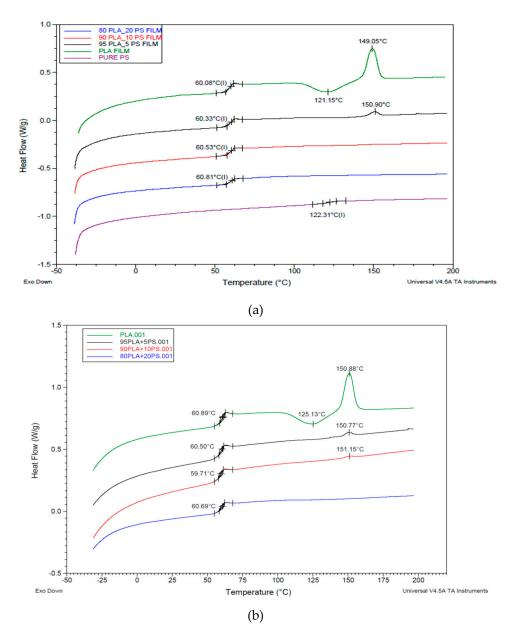
**Figure 4.** Comparison between the second heating thermograms of the **(a)** PLA/acrylic copolymer-based product (PS) cast films; **(b)** PLA/PS cast films treated for 2 min at 190 °C. Exothermal peaks are directed down.
