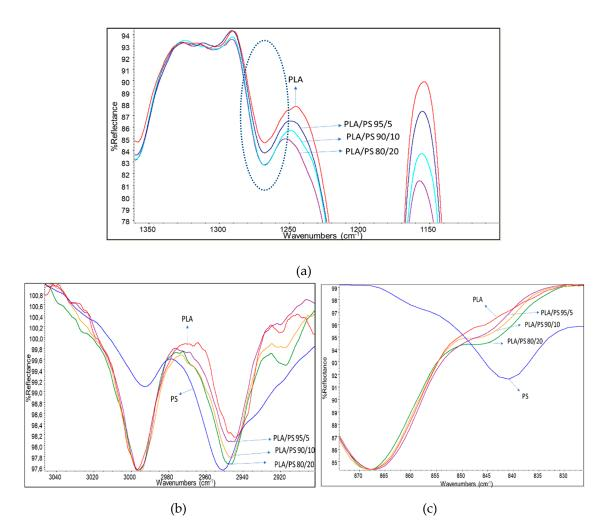
Figure 2. (a) zoom onto the amorphous band of PLA; (b) C-H stretching region of the spectra; (c) rocking  $CH_2$  band (typical of poly(methyl methacrylate)—PMMA) region of the spectra. Spectra were slightly shifted on the vertical direction for normalizing with respect to reference bands, so the reflectance intensity is expressed in arbitrary units.
