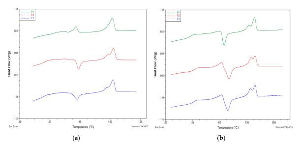
**Figure 6.** DSC heating thermograms of F1, F2 and F3: (a) First heating; (b) second heating. Exothermal peaks are oriented down.
