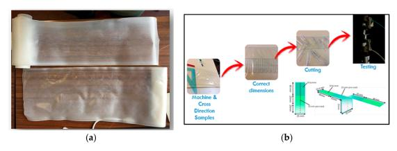
**Figure 9.** (a) F3 semitransparent films obtained by flat die extrusion; (b) methodology adopted for trouser tear tests.
